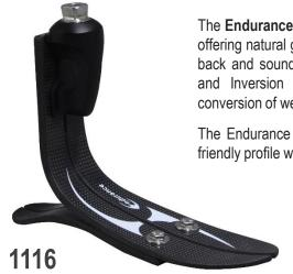
The **Endurance** provides a combination of comfort and dynamics to users offering natural gait with less fatigue and ultimately less strain on the lower back and sound side. The split keel and heel design enhance Eversion and Inversion compliance. The Carbon fiber construction promotes conversion of weight bearing energy input into energy output.
